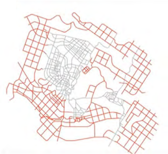
Plan of arterial grid in preparation for the growth of the city of Mekele by 2050 Image source: A new plan for African cities, The Ethiopia Urban Expansion Initiative
